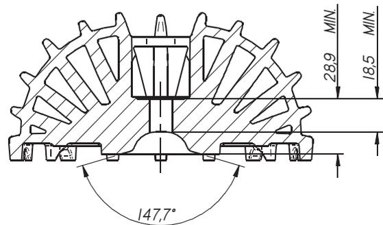
VOLUME CAMERA DI COMBUSTIONE = 7,8 cm<sup>3</sup> MIN.
