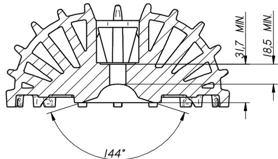
VOLUME CAMERA DI COMBUSTIONE = 10,9 cm<sup>3</sup> MIN.
